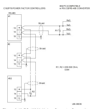
Figure 2-16 RS-485 Multi-drop Computer Connection
