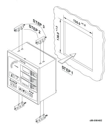
Figure 2-1 Mounting the C191HM
