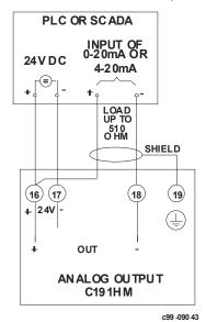
Figure 2-11 Analog Output Connection
