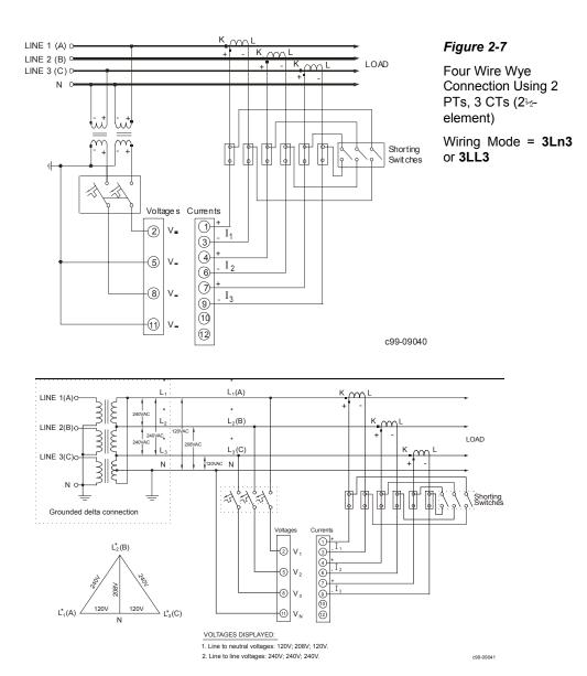
Figure 2-8 Four Wire Delta Direct Connection Using 3 CTs (3 element)
