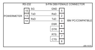
Figure 2-15 RS-232 Simple 3-Wire Computer Connection, 9-pin
