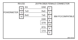
Figure 2-14 RS-232 Simple 3-Wire Computer Connection, 25-pin
