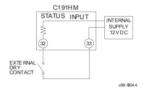
Figure 2-10 Status Input Connection
