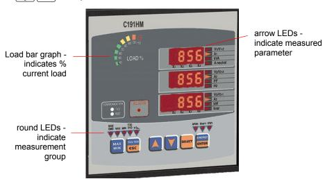
The front panel display is updated approximately twice per second; you can adjust the display update rate via the *Display Setup Menu* (see Section 4.8).
